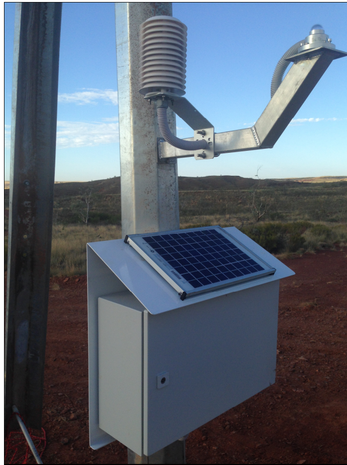
Figure 5 – Temperature, RH and Solar Radiation sensor mounting at Nullagine AWS
