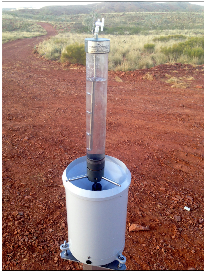
Figure 3 – Tipping Bucket Rain Gauge during field calibration
