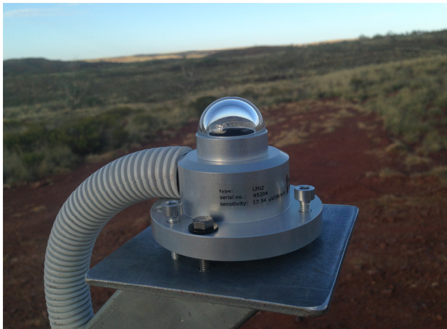
Figure 6 – Hukseflux Solar Radiation Sensor (pyranometer)
